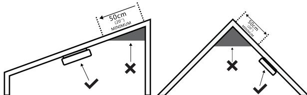
**Note!** If you cannot install the smoke alarm in the ceiling it can be installed on a wall, but it will take longer for the smoke alarm to react to potential danger. Placement needs to be 15 cm from the ceiling.
