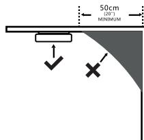
If the ceiling is slanting, the alarm needs to be installed at least 50 cm away (100 cm recommended) from the highest ceiling point in the room.
